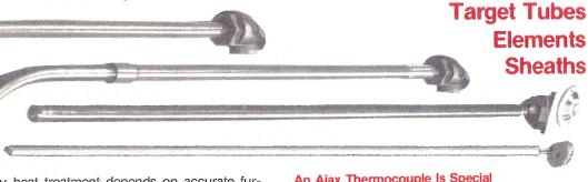
Quality heat treatment depends on accurate furnace temperature. The thermocouple is the most vulnerable part of the temperature measuring system, and therefore thermocouples must be properly designed, fabricated of the best materials, and, of course, accurate.
