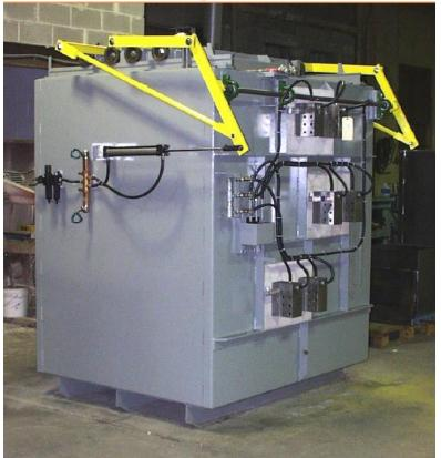
With Ajax HCSE-HHSE ceramic pot salt bath furnaces, your processed steel parts are protected with proper rectification from oxidation, pitting, and decarburization. There's no need for atmospheres, eliminating the need for gas generators or vacuum pumps. The load is further protected by a thin film of salt when being transferred to quench.
